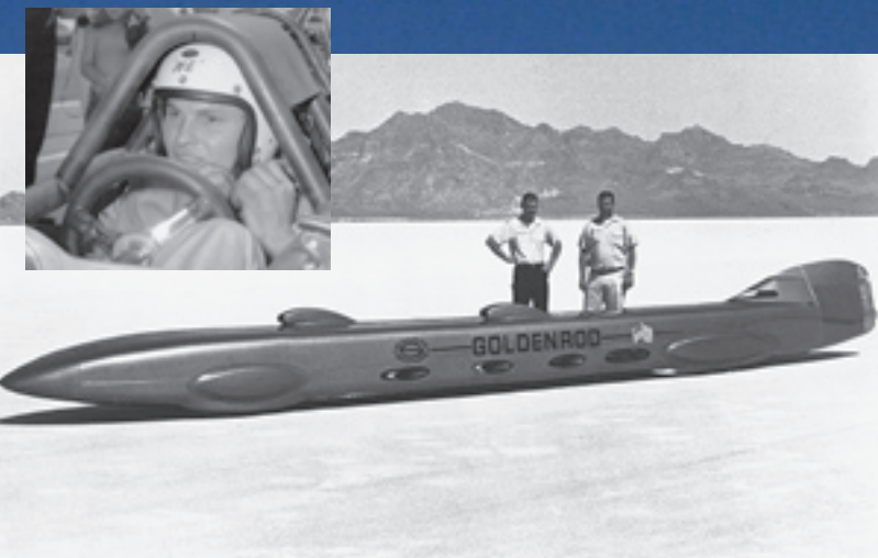
Bob (L) and Bill Summers with the Goldenrod, powered by four 426 Hemi engines supplied by Chrysler. They took the land speed record from Donald Campbell in 1965. Inset photo shows Bob Summers strapping in for a run. The car's restoration was completed last year, and Chrysler again donated the Hemi engines. The Goldenrod is now on display at The Henry Ford in Dearborn, Mich. (Inset photo: The Henry Ford)
